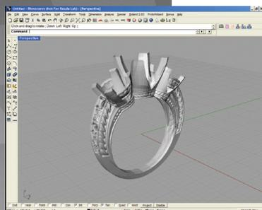
Optional ProtoWizard CAM software steps you through the model making process.
